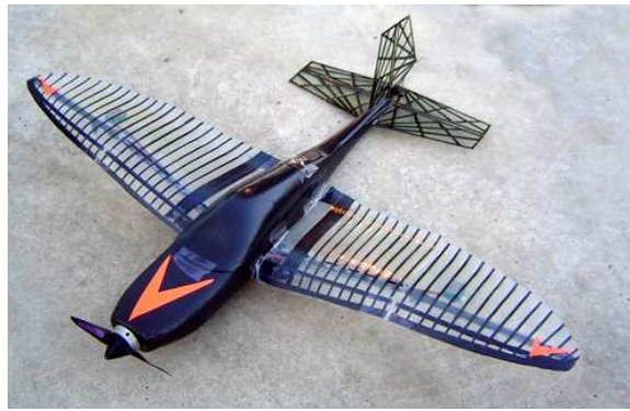
Figure 1. Variable gull-wing morphing vehicle
