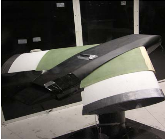
Figure 13. Experimental model mounted in Stability Tunnel
