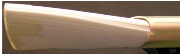
Figure 5. Linear twist distribution due to internal actuation
