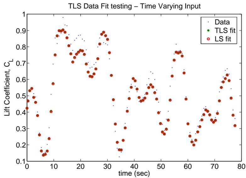
Figure 7. Model Validation : time varying input with large stalling periods
