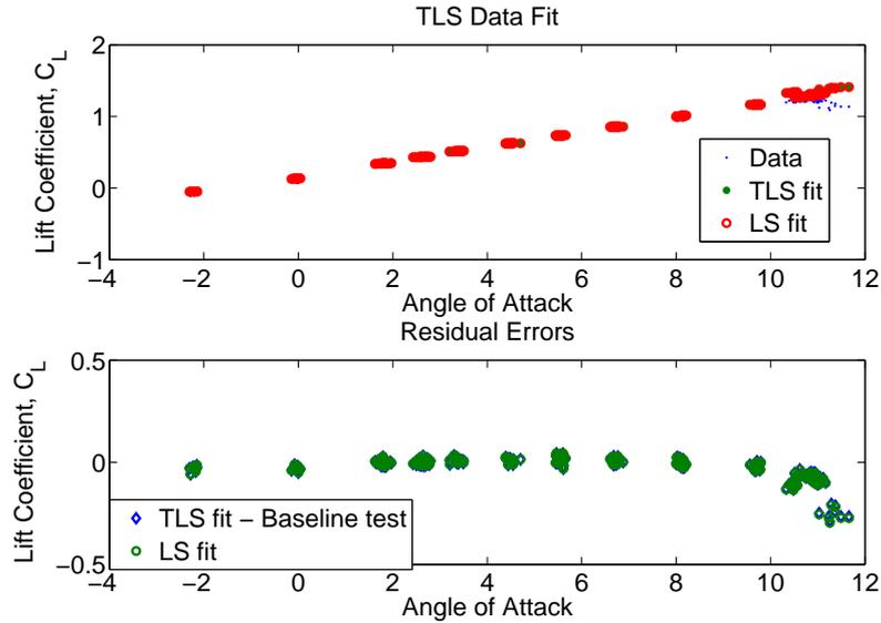
Figure 5. Baseline (no twist) test : Linear Model and Residuals
